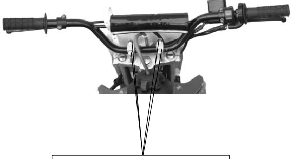
6. Install handlebars by handlebar clamp provided. Torque bolts to 25Nm (18.5ft.lb.)
