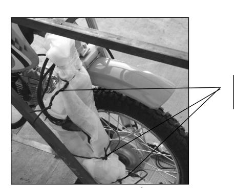
2. Remove wire straps and foam covering from handlebar.
