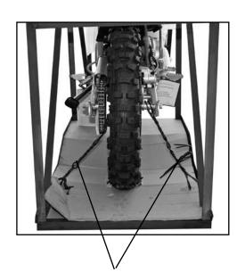
3. Remove wire straps from front forks and rear swing arm.
