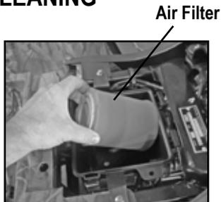
1. Locate Air Filter Box under seat and remove cover.
