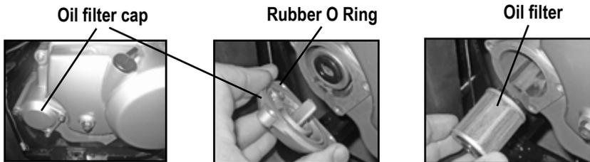
6. Clean oil strainer and oil filter with solvent.
