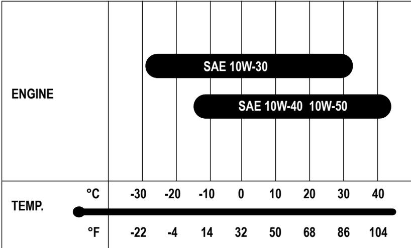
Use the chart to select a viscosity rating based on the temperature range in your area.
