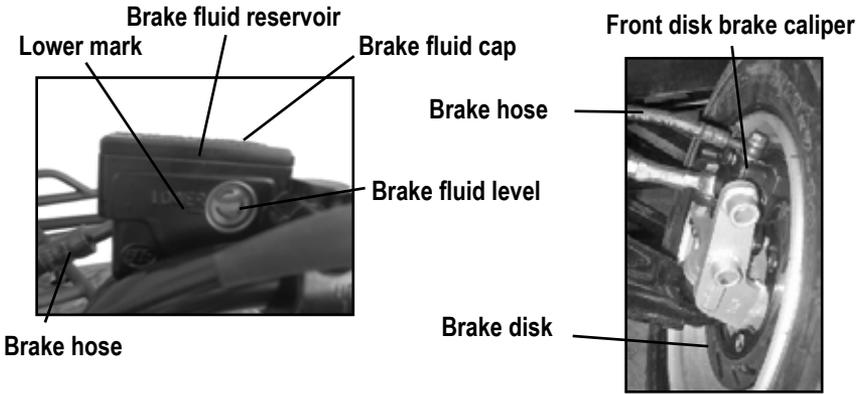
1. Inspect the front disk brake caliper and brake fluid reservoir for leakage. If brake fluid leaks, the safety of riding could be affected.
