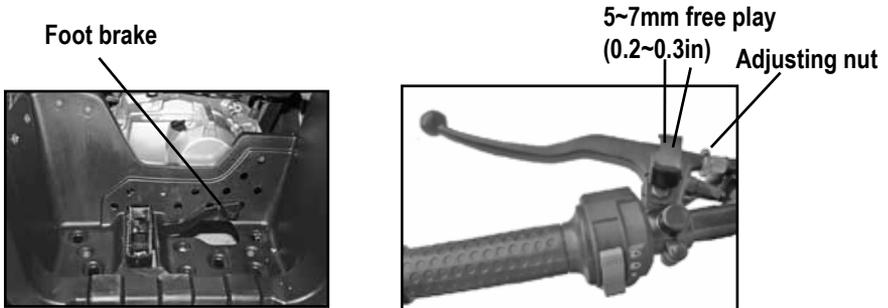
Rear foot brake located on right side of ATV
