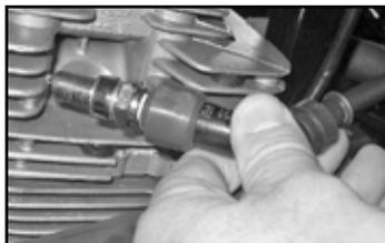
2. Apply the rear brake lever to make sure the rear wheels are locked. Turn ignition key to the “ON” position. Slide the engine stop switch to the “RUN” position. Push the electric button “START “(yellow button). If the ignition system is operating properly, a blue spark should jump across the spark plug gap. If there is no spark, take your machine to your service center.
